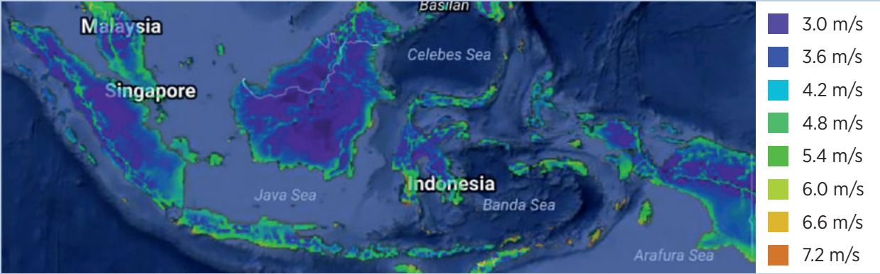
Figure 34: Global wind dataset – 5 kilometre onshore wind speed at 80 metre height with units in metres per second
