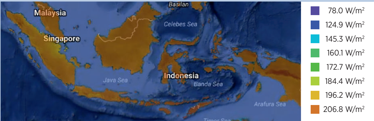
Figure 35: Global solar dataset – 3 kilometre with units in watts per square metre
